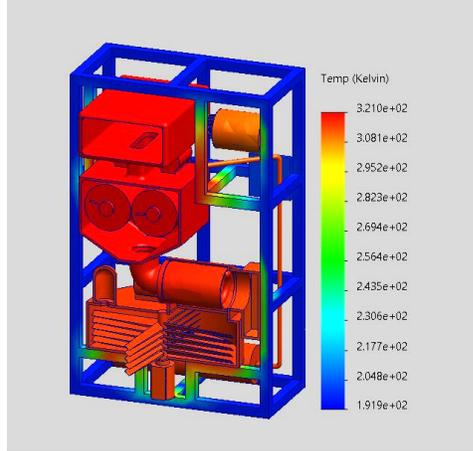
**Figure 10.** SolidWorks thermal model of the payload cross-section
