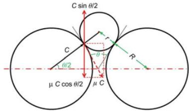
**Figure 7.** Roll Wheel Geometry
