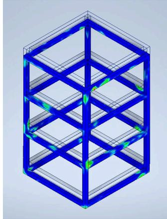
Figure 9. Finite Element Analysis of the payload structure
