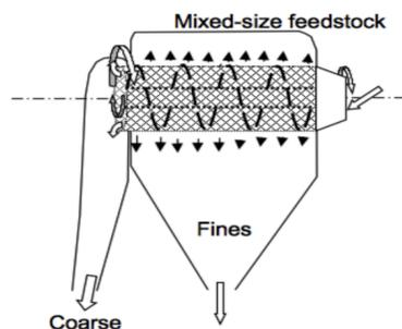
**Figure 8.** Centrifugal Sieve Schematic
