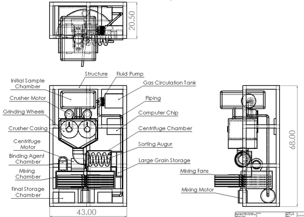
**Figure 2.** Payload 3-View Drawing Annotated (cm)
