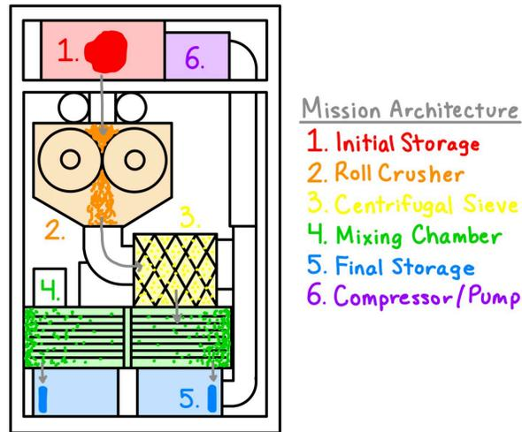
**Figure 4.** Payload Mission Architecture
