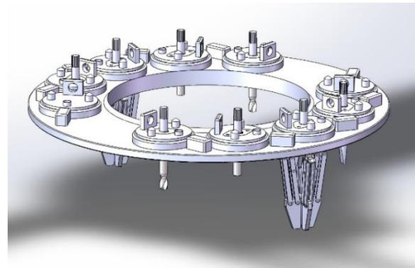
Figure 8: 3D model of the tool holder which will house all 10 tools for the robotic arm.
