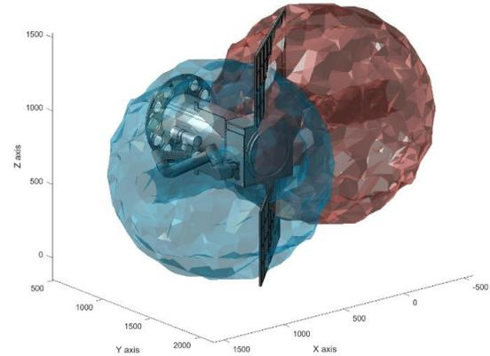
Figure 9: Forward kinematic analysis of the range of motion for both arms.
