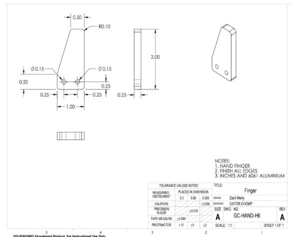
Figure 10: This is a part drawing of the fingertip of the robotic hand. Used as an example of the part drawings that will be used for manufacturing.
