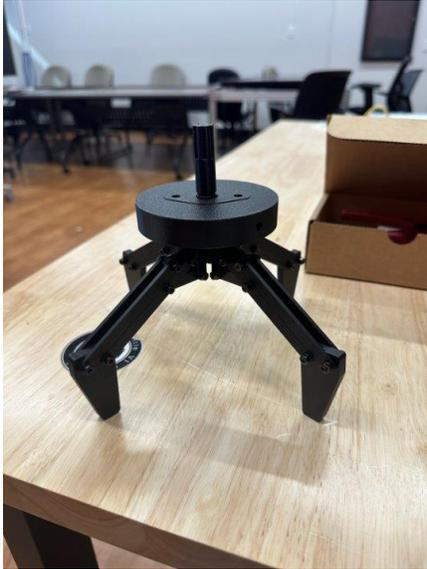
Figure 5: Bottom top view of 3D printed hand at a different claw position to show grip movement capabilities.
