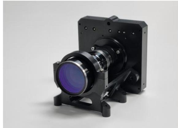
Figure 6: Image of the camera that is planned to be used with the robotic hand for a visual reference.
