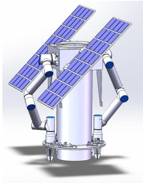
Fig. 2: Full model of Venus class satellite with both robotics arms and hand along with tool holders
