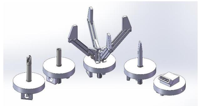
Figure 7: 3D model of the robotic arm and all of the of modular tool examples that the arm is capable of manipulating and completing operations using.
