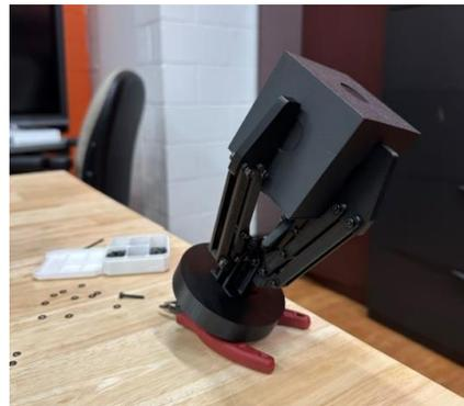
Figure 5: View of the 3D printed hand prototype gripping a 70 mm cube to display its ability to grip small CubeSats.
