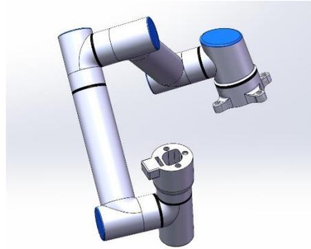
Fig 3: SolidWorks CAD model of the arm disconnected from the bus and the tools.
