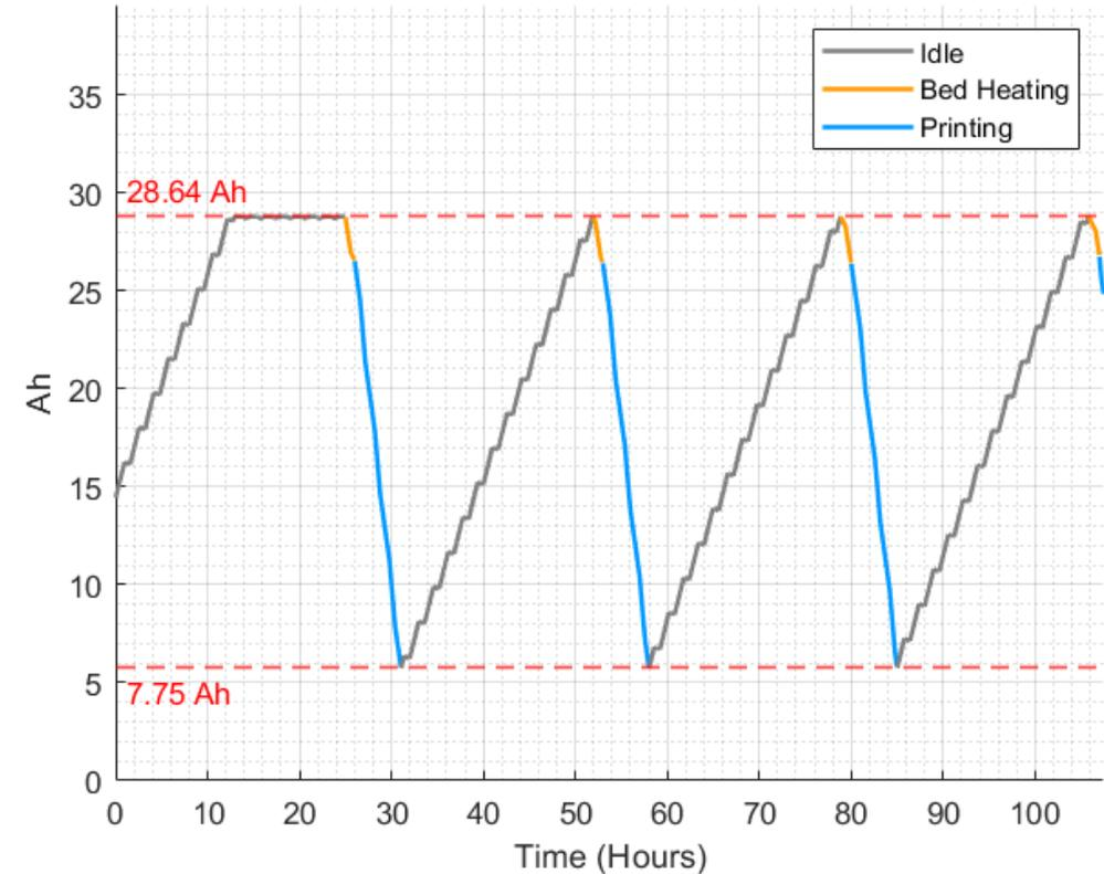
**Predicted Power Timeline for a 3 Inch Print.** The power draw of the fabrication subsystem during a print cycles between a charging phase up to 28.64 Ah (80%) battery storage followed by a discharge down to 7.75 Ah (20%) battery storage during voxel deposition. Ridges in the charge cycle are caused by eclipsing from the Earth. The time to print a 3" tall cylinder is estimated to be approximately 107 hours (70 orbits), with the first 24 hours allocated for idle charging.
