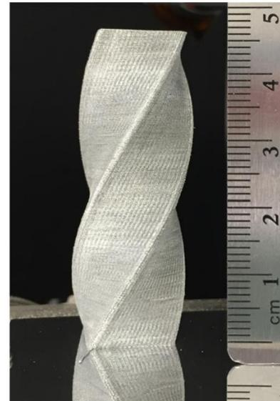
**DAED Additive Manufacturing.** The DAED AM process is demonstrated in the video by the ASU School of Manufacturing, Systems and Networks to the left. Wire feedstock is deposited and compressed by a vibrating toolhead to form a voxel in the build area. The finished product of this print is shown to the right [15].
