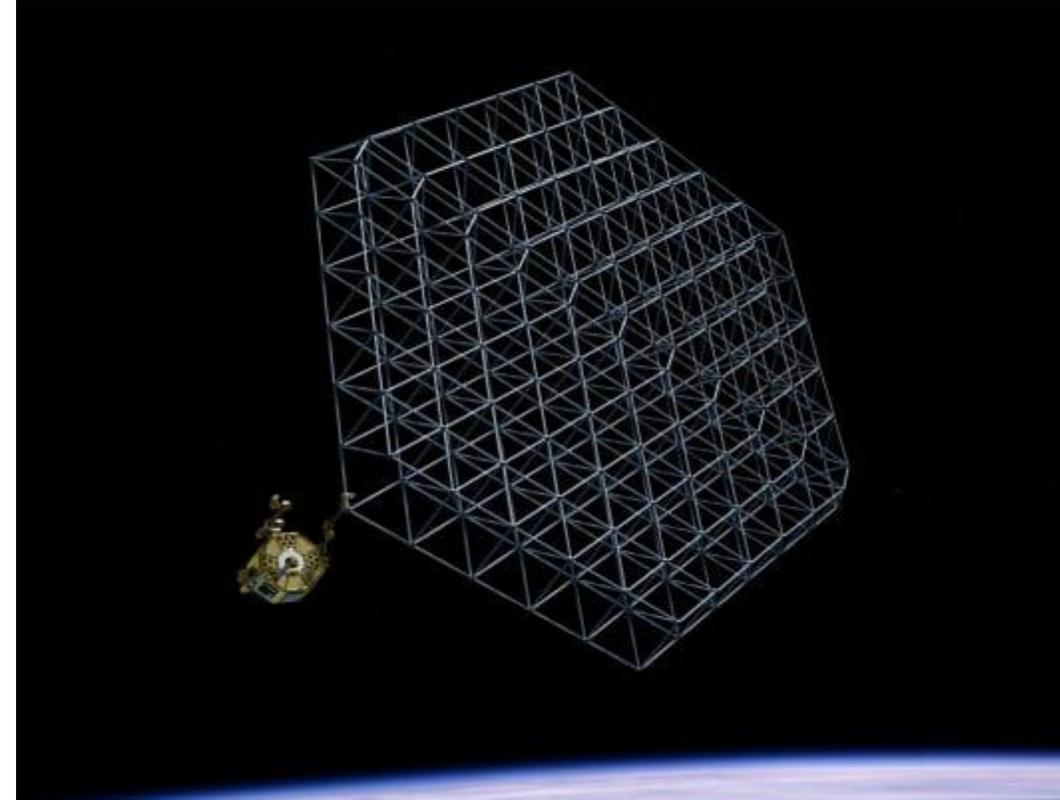
**Concept of In-Space Structural Fabrication.** Demonstrating the ability to fabricate and assemble structures in space would enable future missions to manufacture large structures without the restrictions launch puts on modern space vehicles. This concept art was developed by Made in Space [7].
