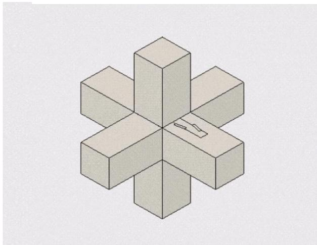
**Traditional East Asian joint method.** Traditional East Asian joint assembly was considered for in-space structural assembly early in concept development. It was not pursued due to the precision required to join the pieces together [3,4].
