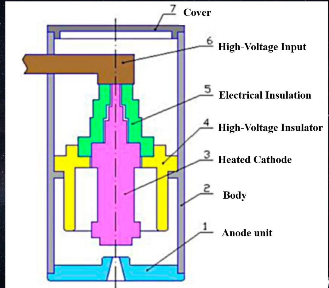
Image from Paton et. Al. , "New Electron Beam Gun for Welding in Space," , *Science and Technology of Welding and Joining*, Vol. 24, No. 4, 2019, pp. 320–326. <https://doi.org/10.1080/13621718.2018.1534794>
