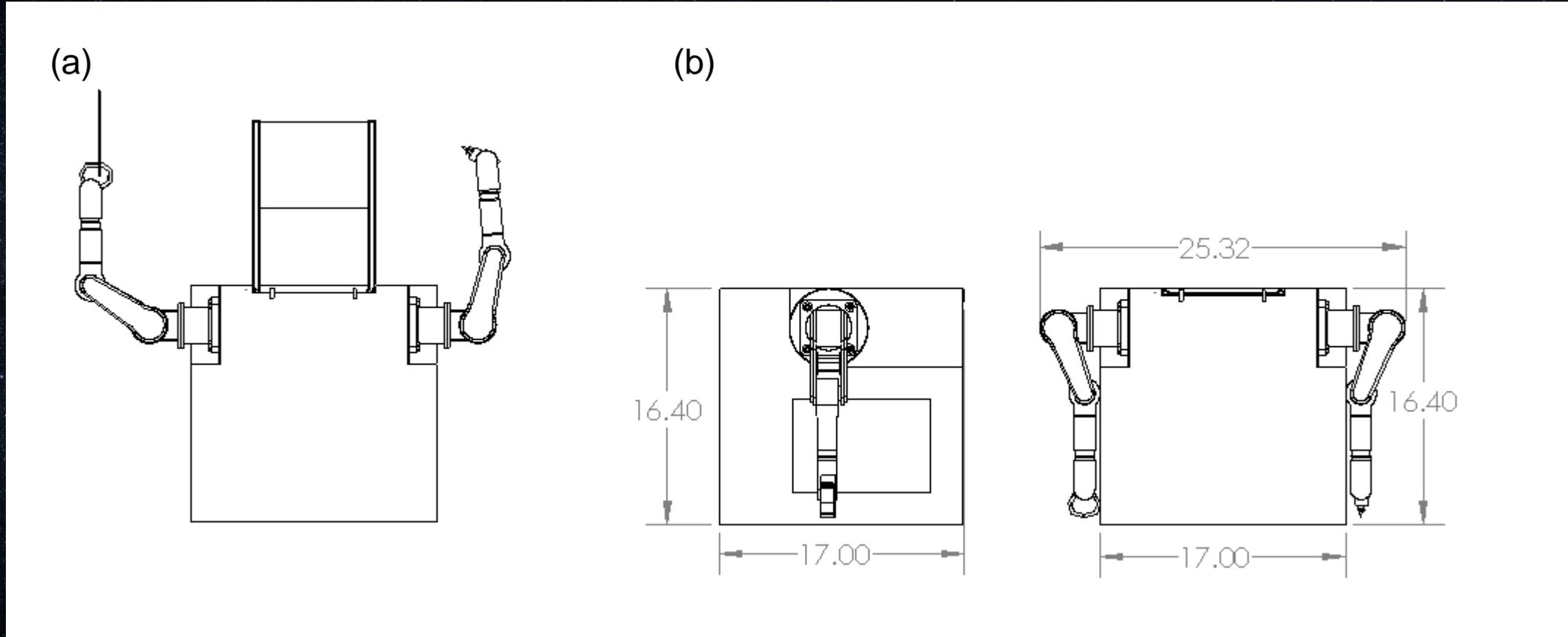
**Final Design: (a) payload configuration once deployed and in use (b) payload configuration for launch (dimensions in inches)**
