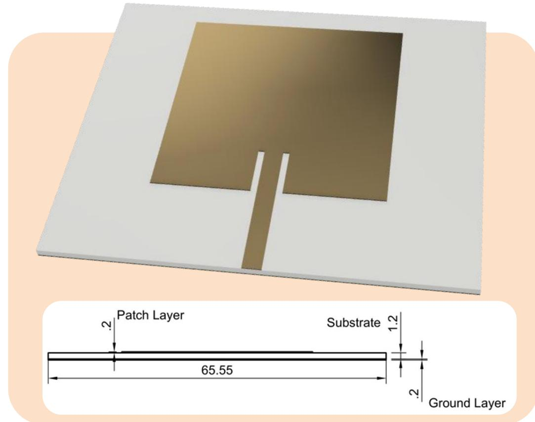
Patch antenna to be manufactured by the payload
