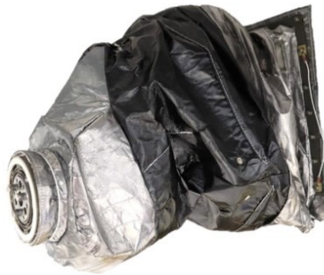
Fig. 11 "Socks" Found on the VIPER Rover Preventing Dust Damage [27]
