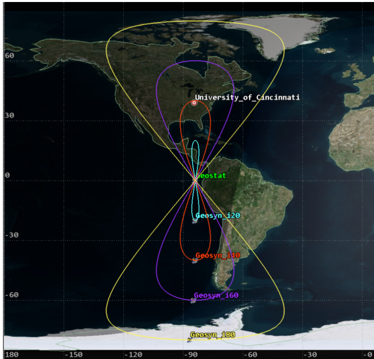
Fig. 1 Possible Geosynchronous Orbits, with No Eccentricity and Varying Inclinations
