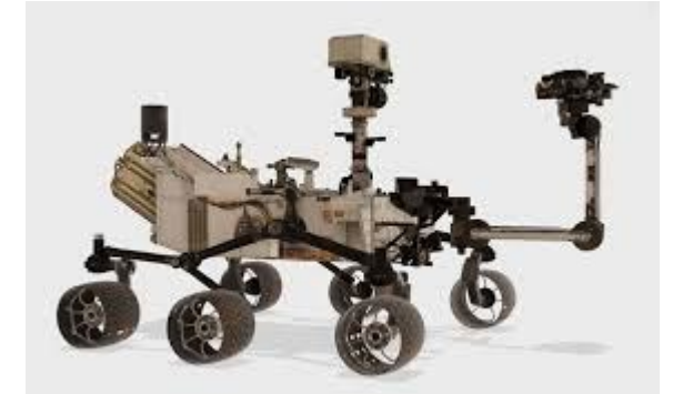
Curiosity is a Mars rover that uses rocker-bogie suspension [33]
