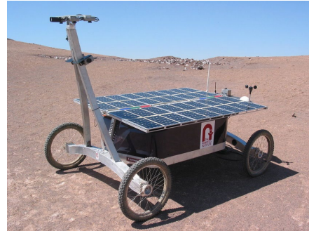
Zoë is a single-rocker rover designed by Carnegie Mellon researchers [31]
