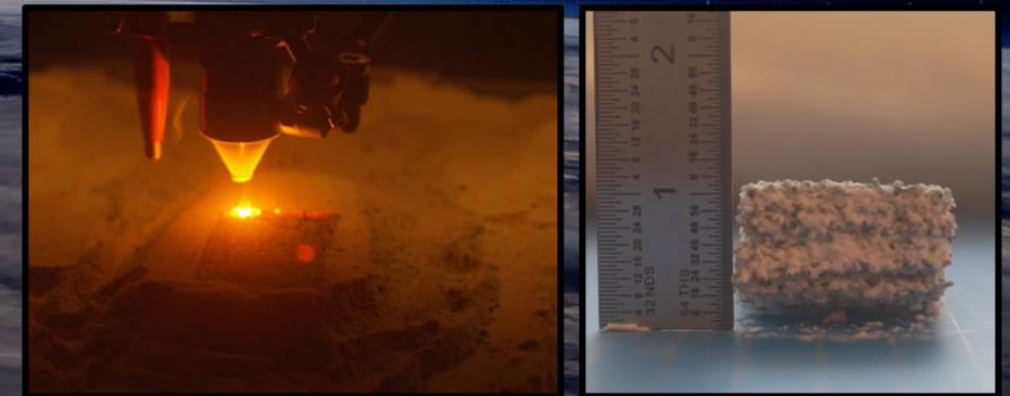
Sintering Achieved with 150W Laser
