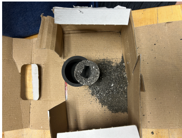
Figure 5: Clump of melted sand on crucible
