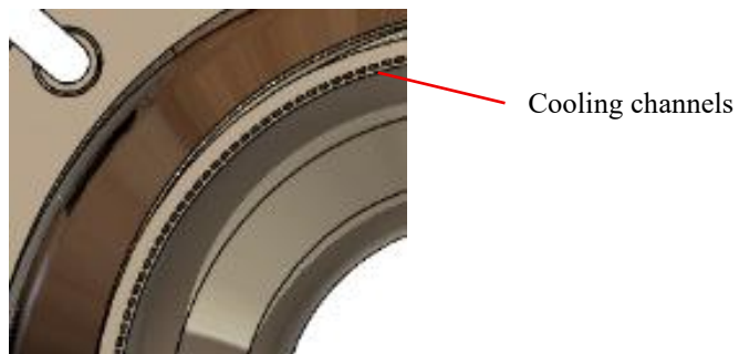
Fig. 7 Janus R Regenerative Cooling Channels
