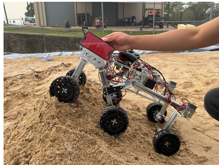
Slope Longitudinal Tilt - PASS
