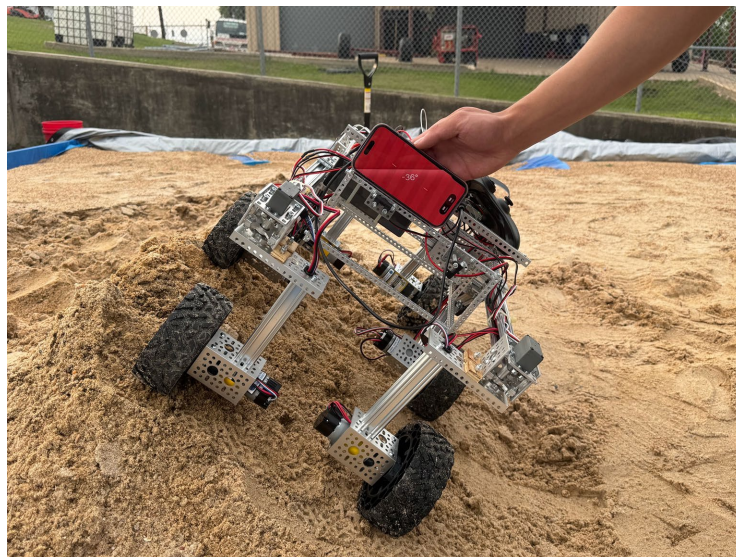
Slope Lateral Tilt - PASS
