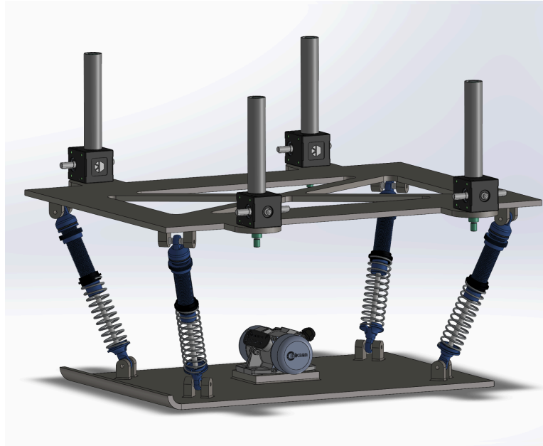
Figure 8: CAD Model of Plate Compactor and its Connection to the Chassis
