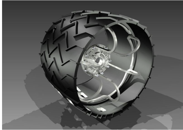
Fig. 8 Skeletal aluminum rover wheel with integrated grousers and reinforced hub structure.
