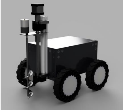
Fig. 1: Aurora Auger concept, used for gathering various depths of He-3 for direct measurements.
