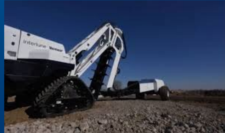
Figure 2. Full-scale prototype of the Interlune helium-3 excavator, developed in partnership with Vermeer. Source: Interlune 2025
